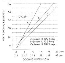
\*Heat load removal depends on the temperature of your in-house, or tap water system. We've plotted the cooling capacity based on a 10°C temperature differential (Δ1°C) between your supply water and the water at the System III outlet. Pressure differential required from house water system does not exceed 10 psi.
