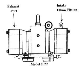
Warning! Remove Plug From Exhaust Port Before Operating
