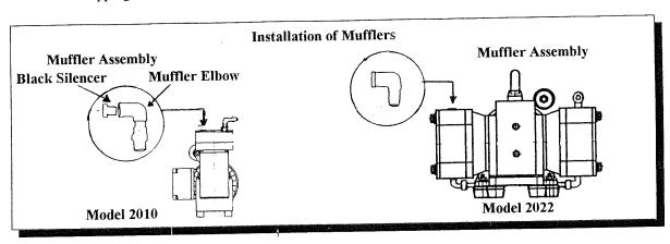
Since Model 2015 has two exhaust ports, two mufflers are provided. The mufflers are installed on the exhaust ports of the pump.
